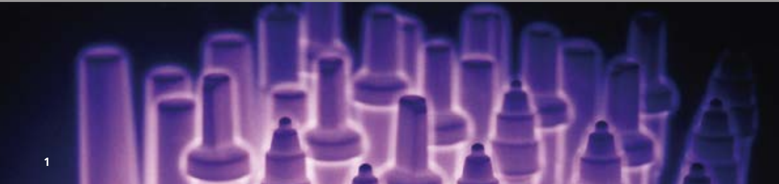
1 Diecasting cores during plasma nitriding.
