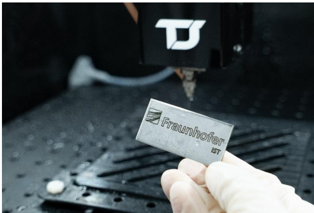
Fig. 2 Local surface structure on a stainless steel substrate created by electrochemical jet machining (EJM). © Fraunhofer IST
