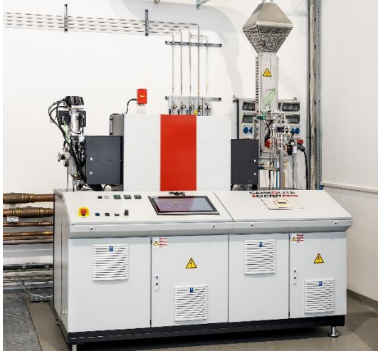
Fig. 2 The recently available high-temperature furnace enables investigations in the temperature range of up to 1,600 °C. © Fraunhofer IST
