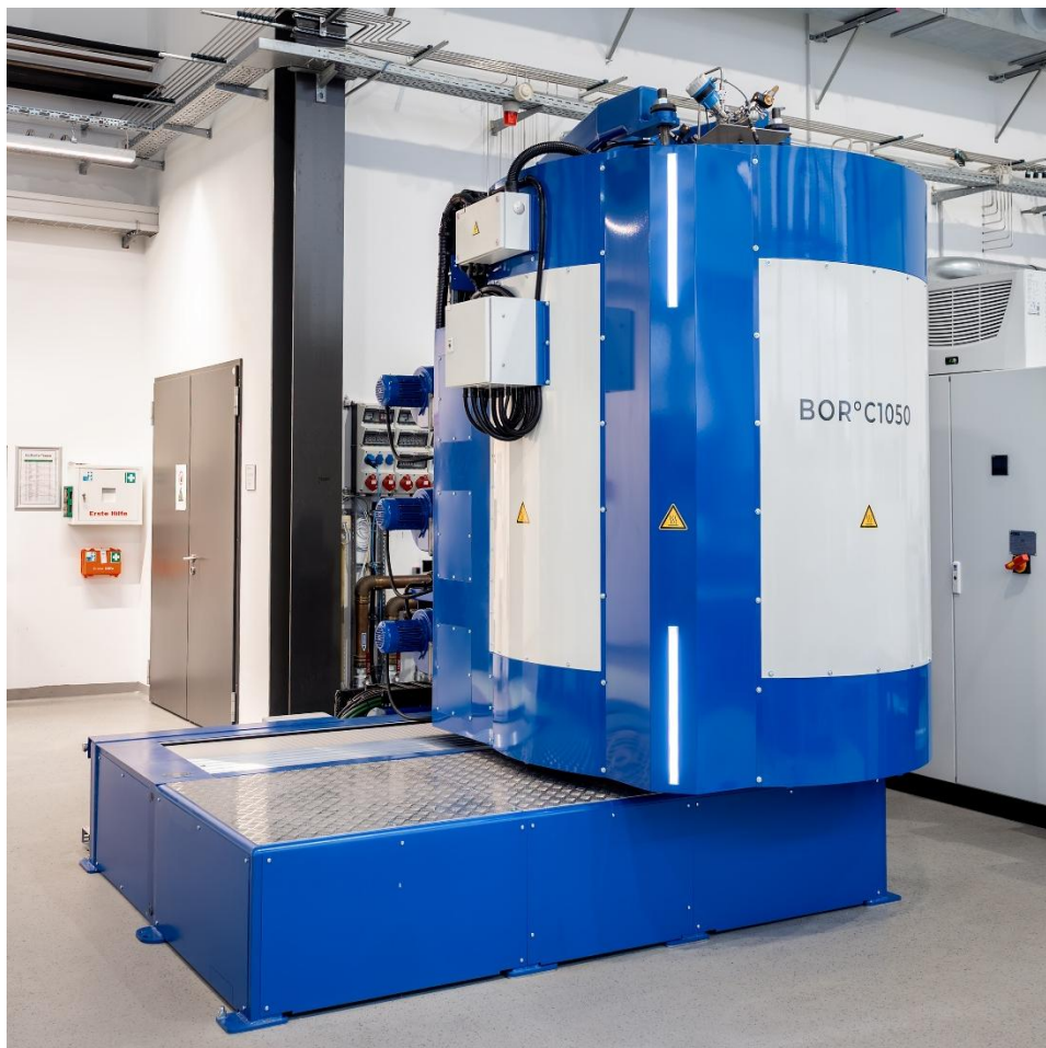
Fig. 1 The new gas boriding plant at Fraunhofer IST uses diffusion treatments at temperatures of up to 1,050 °C to create boride boundary zones with exceptional technological properties. © Fraunhofer IST
