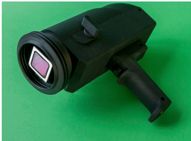
Demonstrator of a mobile measuring gun with luminescent polymeric carrier.
