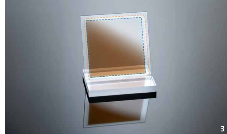
3 First prototype of an electrochromic emittance modulator; the dashed lines indicate the location of the respective contact layer.
