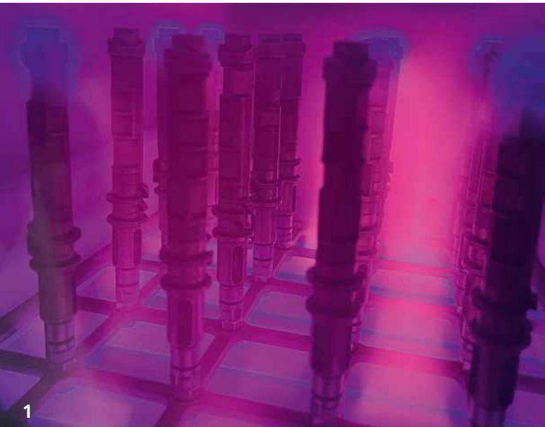
Components for high-precision bicycle gear systems are coated in a plasma environment using the COAD® process.
