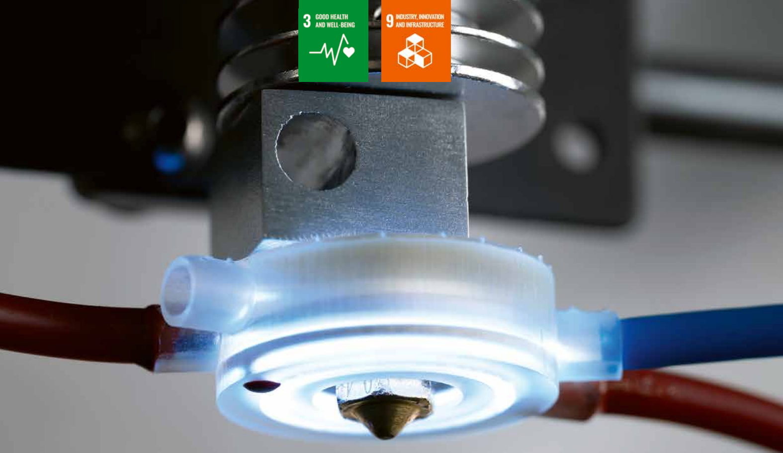
In-situ plasma coating during 3D printing: A plasma ring source developed at Fraunhofer IST generates reactive bonding sites on the polymer surface directly during the extrusion process.
