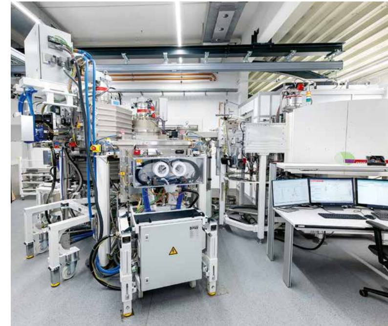
OPTA X coating system (by Ardenne) featuring our second-generation EOSS® technology for simultaneous deposition on both sides of interference filters.
