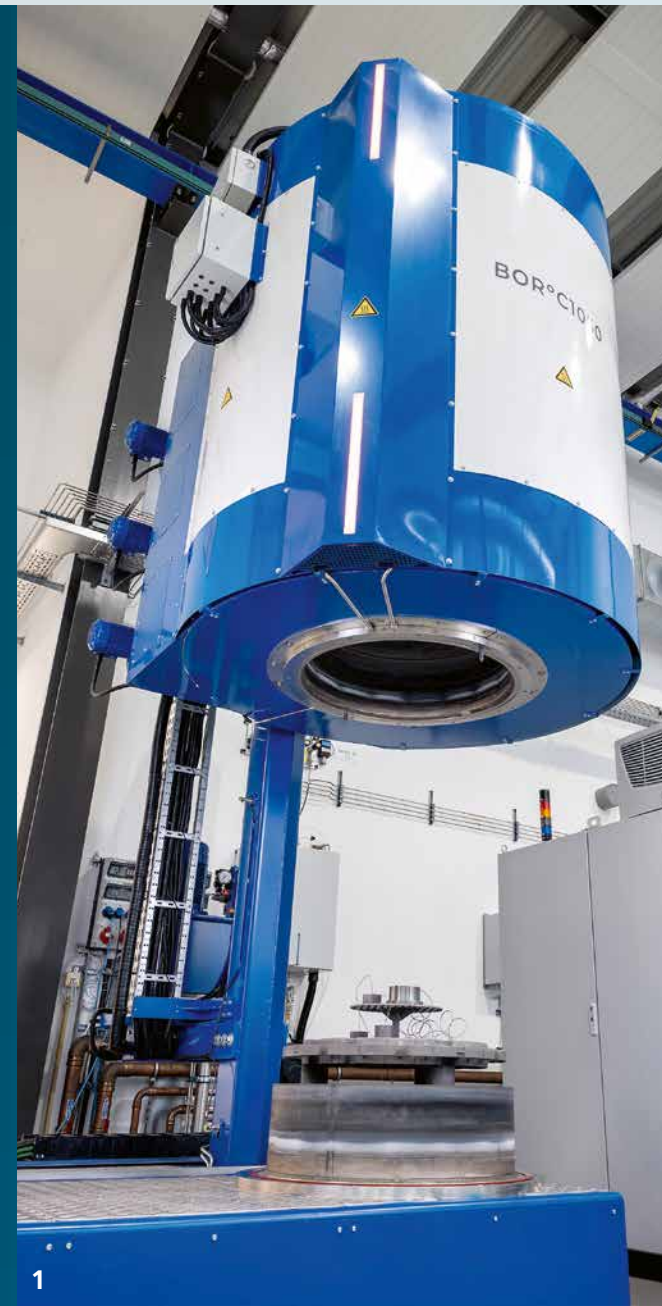
The new gas boriding plant at Fraunhofer IST uses diffusion treatments at temperatures of up to 1,050 °C to create boride boundary zones with exceptional technological properties.
