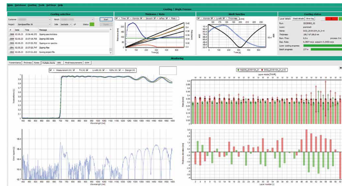
Process control at an industrial plant: MOCCA® user interface during the coating of a cavity filter.
