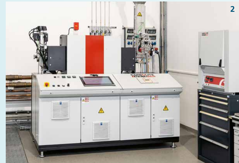
The recently available high-temperature furnace enables investigations in the temperature range of up to 1,600 °C.
