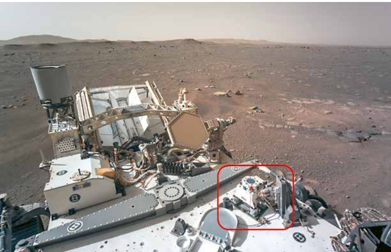
Technology from the Fraunhofer IST on Mars: The interference filter (right) is a component of an optical sensor for dust characterization in the "Mars Environmental Dynamics Analyzer", or MEDA for short.
