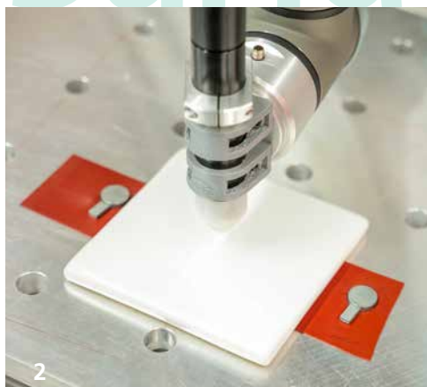
Robot-guided plasma coating of a tile.
