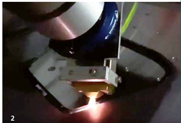
Plasma treatment of three-dimensional surfaces using a robot-guided system.
