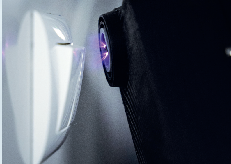
Modular plasma source for the cleaning and disinfection of surfaces.
