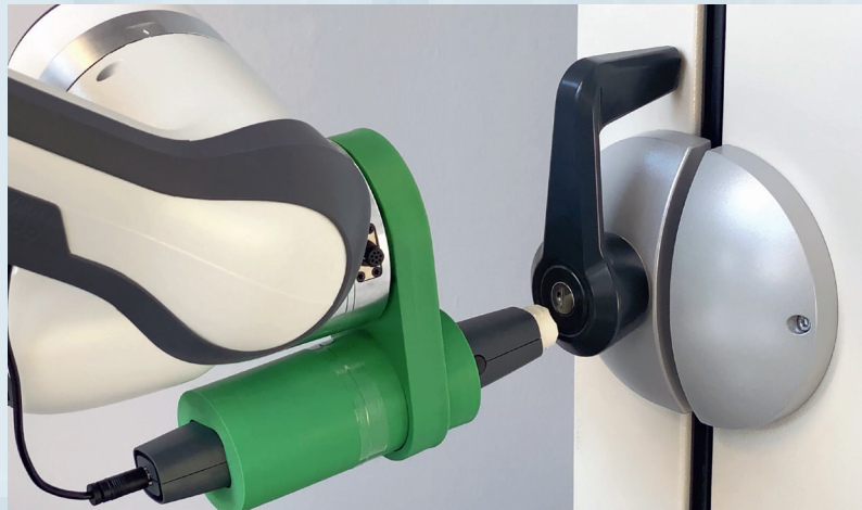
Automated cleaning by means of plasma technology: integration of a plasma source into a robot arm.
