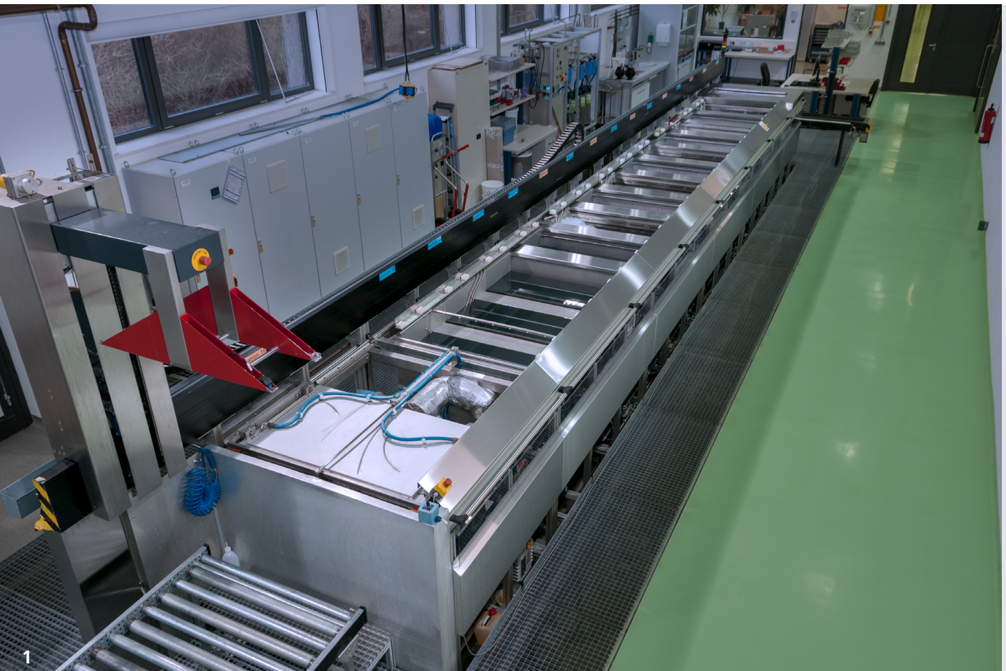
Multi-chamber system for aqueous cleaning at the Fraunhofer IST, with high reproducibility and flexibility with regard to the materials to be cleaned.
