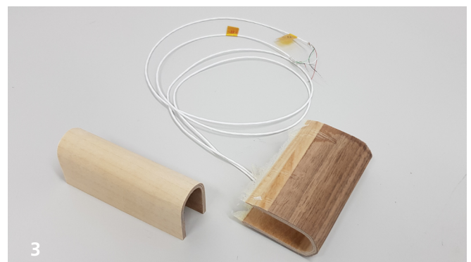
Formed veneer with sensor integration.
