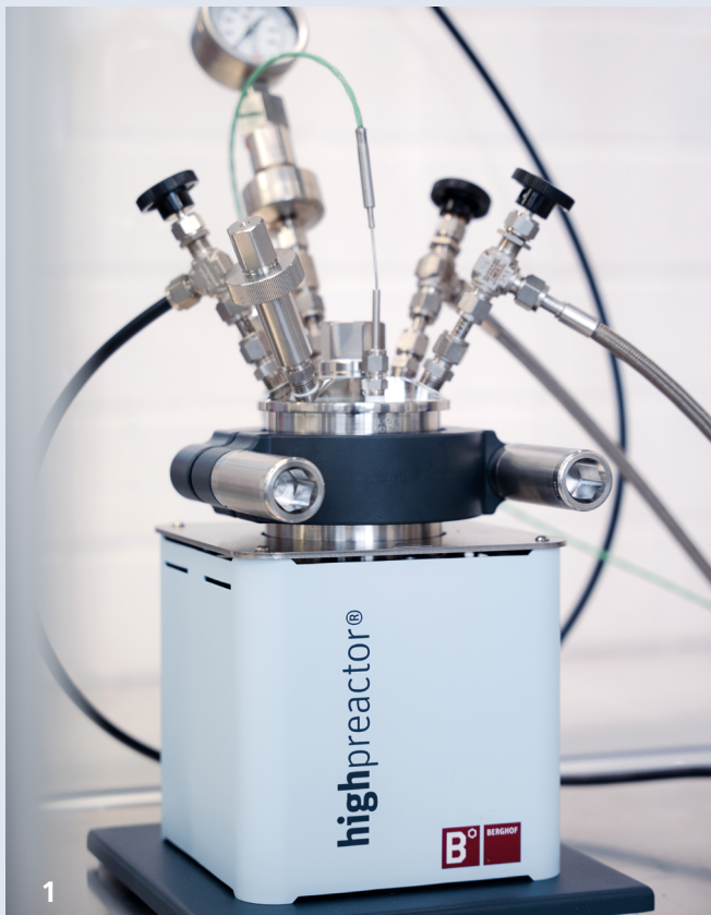
Deuterium reactor for controlled loading of samples with hydrogen or deuterium gas with pressures up to 200 bar and temperatures up to 300 °C.
