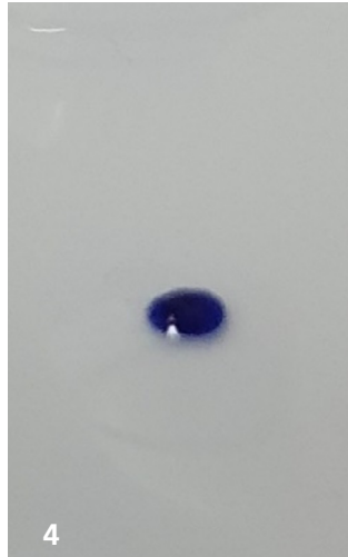
Alteration of the wetting behavior of a PE surface as a result of treatment with the plasma nozzle.
