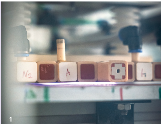
1 As a result of plasma coating, functional anti-adhesion layers are applied within a short time via a dry process control.
