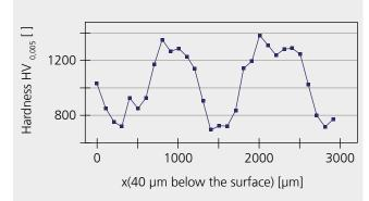
Hardness measurements taken 40  $\mu$ m below the structured surface demonstrate the effects of the covering: Whilst ductile zones form under the covered and thereby untreated areas, nitrided zones form under free areas with a high hardness.
