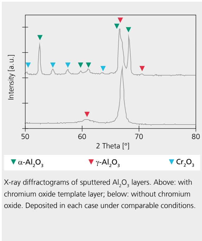
X-ray diffractograms of sputtered  $\text{Al}_2\text{O}_3$  layers. Above: with chromium oxide template layer; below: without chromium oxide. Deposited in each case under comparable conditions.
