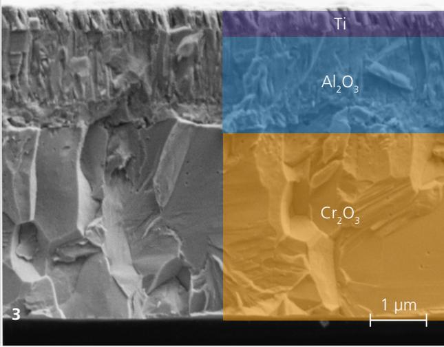
1 Fracture edge of a thermally grown aluminum oxide layer on a high-temperature alloy.
