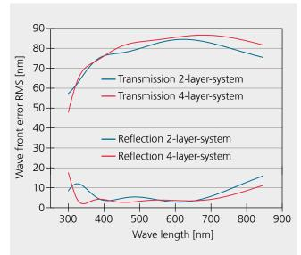
Transmission (above) and reflection (below) for unilateral diamond-based anti-reflective coating systems with two or four sublayers (blue and red lines).
