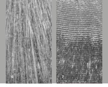
the modification yielded positive benefits. Compared to the series production dies, which have only been gas nitrided, the modified dies showed marked improvements in abrasive wear, especially in tribologically highly loaded areas. Furthermore, an increase in service life was achieved as a result of a considerable decrease in mechanically induced cracks.
