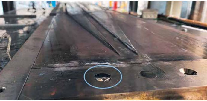
Flat-die tool with integrated sensor insert. 1
